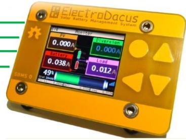
1. Do not put a fuse or breaker (or anything else) between the battery + and the Shunt(s). If the fuse/breaker were to blow, the resulting voltages on the input to the SBMS0 could damage it.
