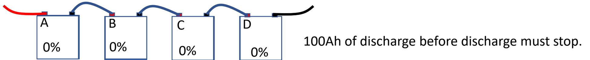
You can also charge the bank with 100Ah before all of the cells are fully charged.
