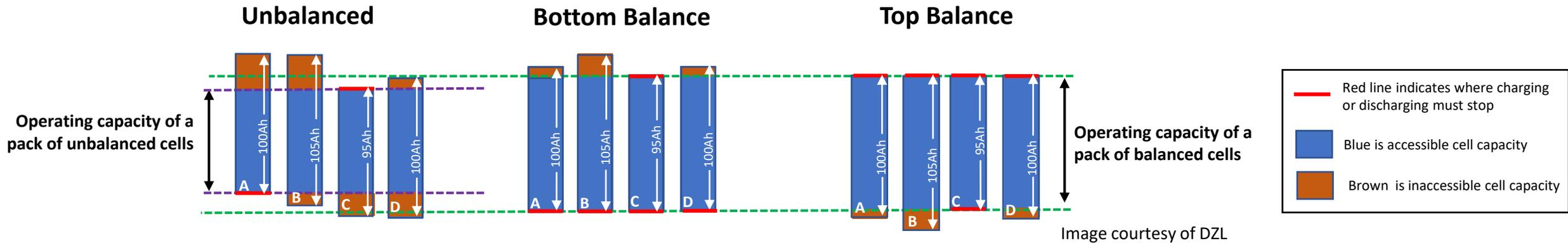
Notice that in the unbalanced case above, the charging must stop when cell C hits its max charge even though A, B & D could still be charged more. Furthermore, discharging must be stopped when cell A hits its minimum charge even though cell B, C & D could be discharged further.
