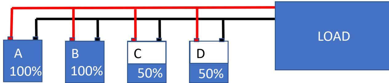
The cells are drained till they reach a voltage indicating 0% state of charge. This is typically done multiple times at different voltages in order to get them all to a target resting voltage.
