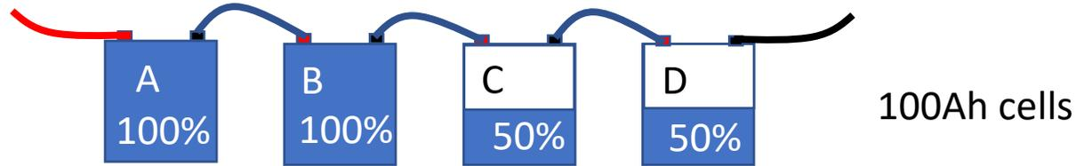
Since cell A & B are fully charged, you can not charge this bank any further without damaging cells A & B. The BMS must stop charging as soon as one of the cell voltage indicates 100% charge for that cell, even though the total battery voltage will be low.
