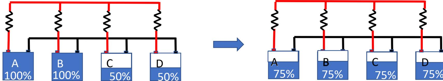
Note: The voltage difference between a fully charged and full discharged battery is only  $\sim 0.5V$ . Consequently, with a 1 ohm resistor, the equalization process can take a very long time.
