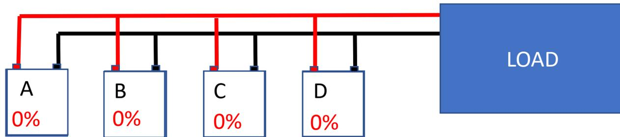
At this point the cells can be put back into a series battery and they will charge and discharge together. Consequently, you will get the max storage out of your battery.
