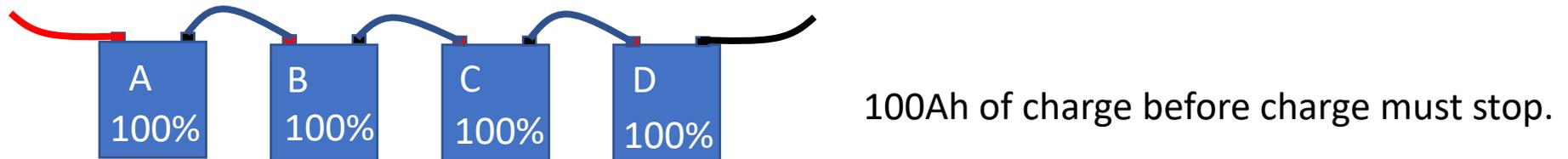
You can see from this example that in order to get the full use of the cells, you need to start with cells that are all at the same state of charge (Balanced).
