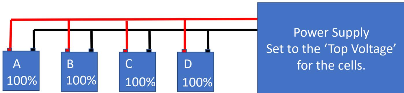
Note: With cells that are way out of balance, you may want to first equalize the cells with resistors before balancing. (See appendix A: Equalizing Cells)
