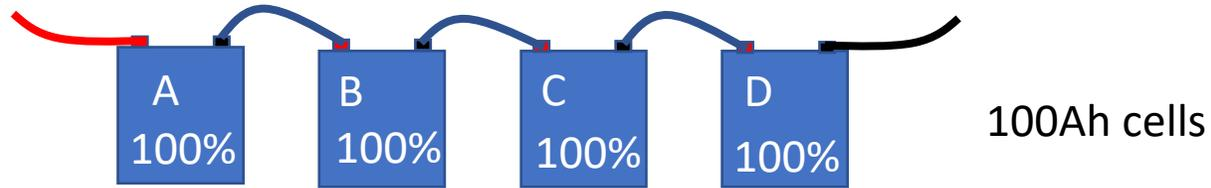
With this as the initial condition, you can drain 100Ah from the battery before all of the cells are empty
