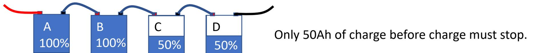
In this extreme example, the battery bank has an effective capacity of only 50Ah even though 100Ah cells were used.
